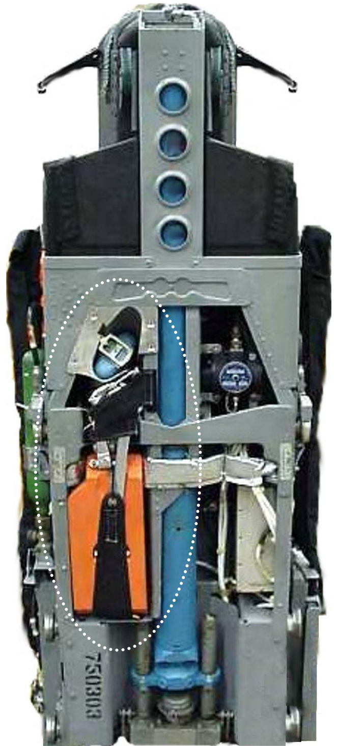
Figure 11. Enhanced Drogue Installation.
