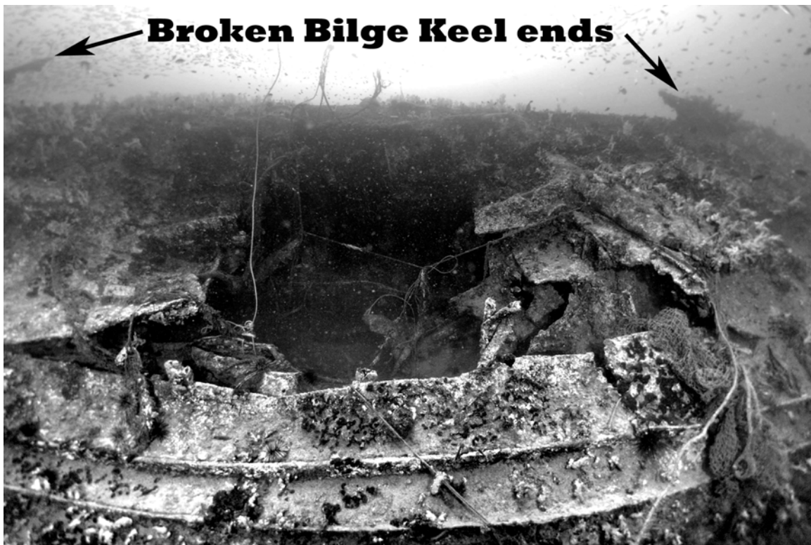
Photo is of the starboard amidships hit on Repulse , which is approx 4m high x 6m wide. Top left and right can just be seen the remains of the destroyed bilge keel. (NOTE; the distortion/curvature seen at the bottom of photo is from the use of a Fisheye - 180° - lens.)
