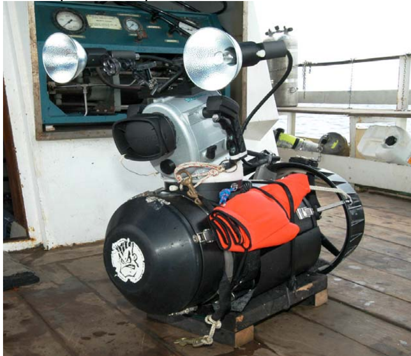
Diver Propulsion Vehicle, with video camera and lights swivel mounted for wreck survey.
