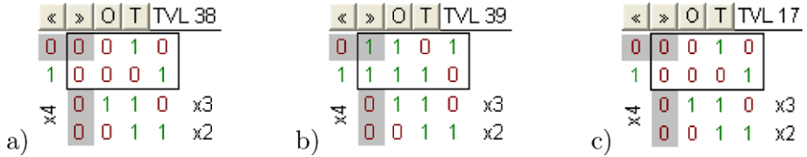
Figure 7.14 Functions on the branch h_2 of the weak OR-bi-decomposition of the function g_1 of Fig. 7.10 a): a) h_{2q}(x_2, x_3, x_4) as object 38, b) h_{2r}(x_2, x_4) as object 39, and c) the realized function h_2(x_2, x_3, x_4) as object 17
