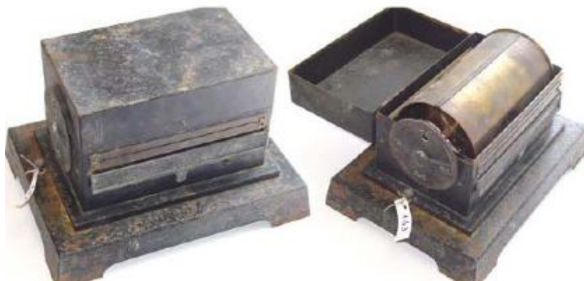
Fig. 14: The photographic system from the Kelvin-Mascart Electrometer (Instituto Geofísico da Universidade do Porto – photograph, courtesy of Marisa Monteiro, MCUP).
