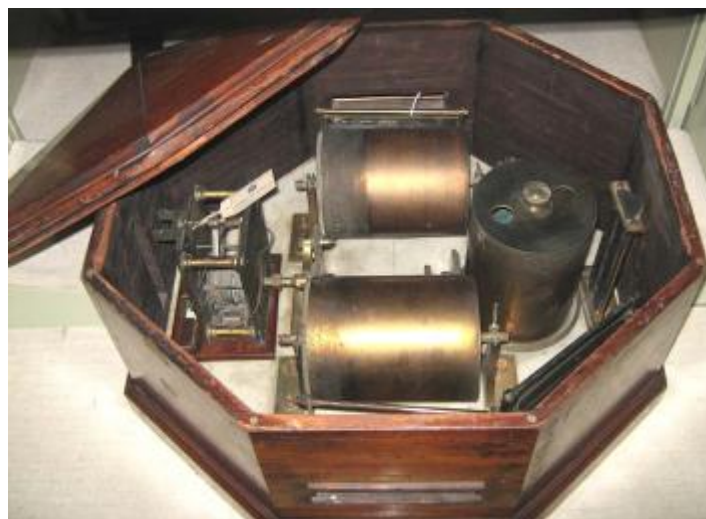
Fig. 16: Octagonal box with devices for registering the magnetographs (MCUL.00354) (Photograph by Marília Peres).
