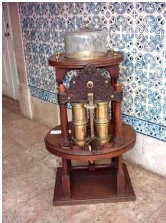
Fig. 5: Pneumatic machine for Leslie Experiments, MCUL153 (Photo: S. Carvalho, Courtesy Museum of Science, University of Lisbon)
