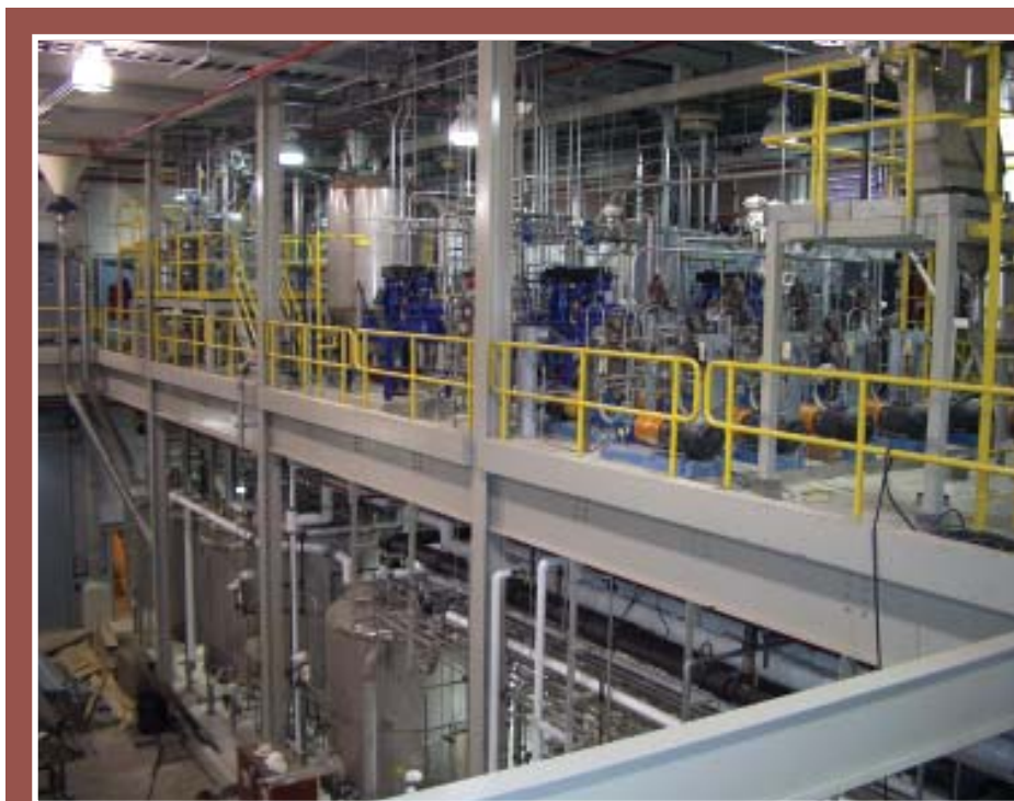
The National Corn-to-Ethanol Research Center emulates both the wet and dry mill ethanol production process. Equipment for the wet mill process is one side of the facility, and equipment used in both processes is on the other.
