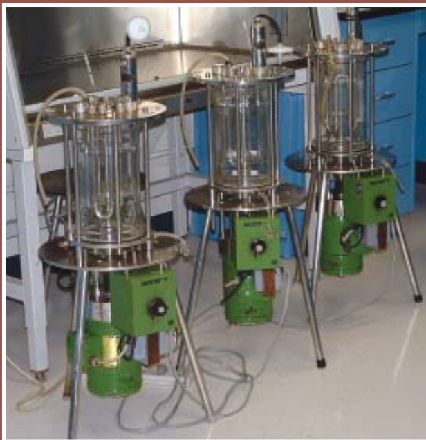
Three of six benchtop fermenters donated by Genencor International. They each have a capacity of 3 to 5 liters.
