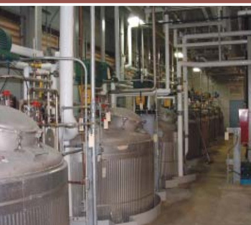
The NCERC’s equipment is the smallest commercially available. The four fermentation tanks have a capacity of 6,000 gallons each.
