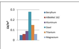
Miinimum gage aluminum applications. Density is approximately the same as fiberglass. AlBeMet<sup>®</sup> can provide weight savings of 25%.
