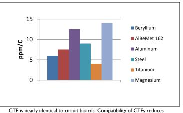
thermal strains between cores & circuit boards. Compatibility of CTEs reduces thermal strains between cores & circuitry components resulting in fewer failures. In an application the CTE of the base material is a dominant contribution to thermal mechanical stress.
