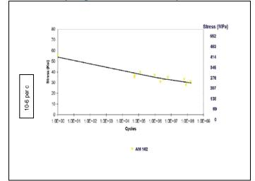
The AlBeMet® Fatigue-Extruded Heat Treated (593°C-24 hr)
