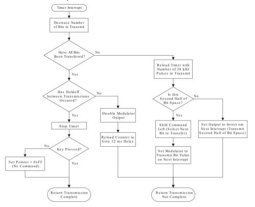
Figure 5-3. Timer Overflow Interrupt Flowchart
