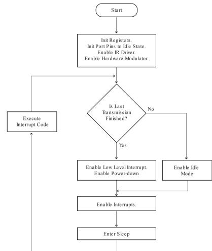
The program execution can roughly be divided into two states; "Transmitting a RC5 code" and "Waiting for a key to be pressed". While waiting for a key to be pressed, the ATtiny28 is put in Power-down mode. In this mode the current consumption for the device is at a minimum, and the wake-up time is slightly longer than for the Idle mode. Since the wake-up condition is caused by physically pressing a key, the longer wake-up time will not cause a noticeable delay in the system.
