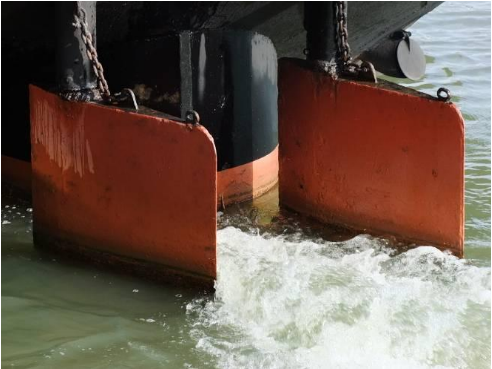
Figure 6.10 Example of a multiple rudder system on an inland vessel
