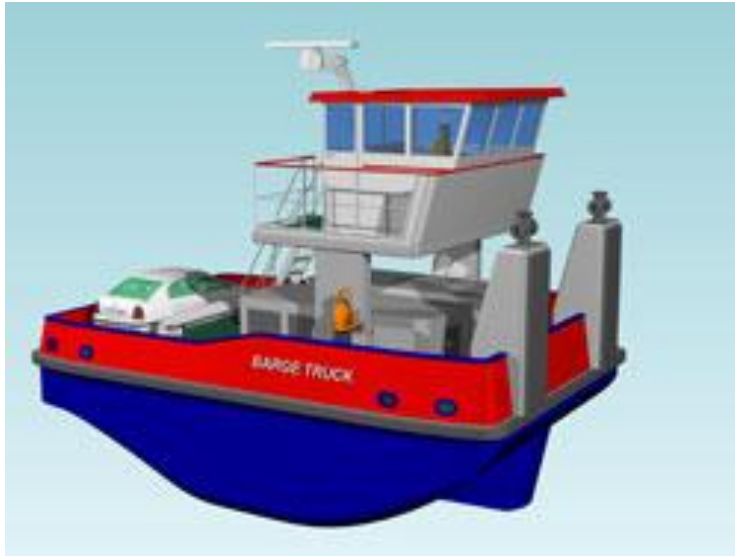
Figure 7.3 Conceptual design of a mini-pushboat for the water truck system
