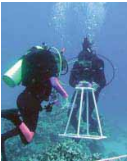
Tool For Quantifying Algae (Linda Preskitt). Research divers using the photoquadrat method to survey reefs.
