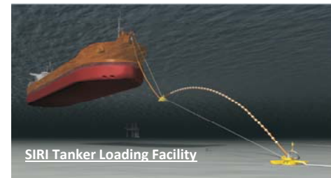
Illustration of hose when idle.
