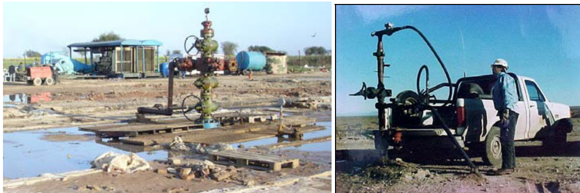
FIG. 111. Tritium injection using bypass technique.
