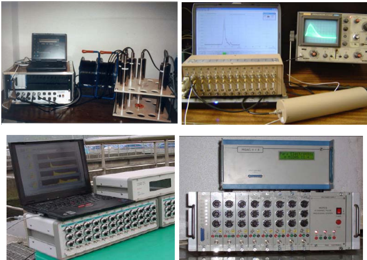
FIG. 22. Data acquisition systems for online radiotracer tests
