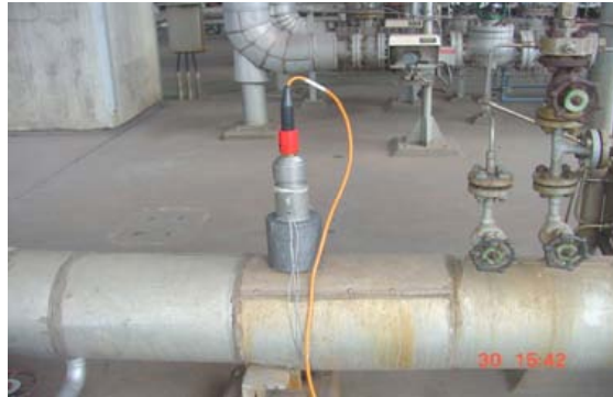
FIG. 16. On-line detection of gamma emitting radiotracer: NaI probe with collimator mounted at the reactor outlet.
