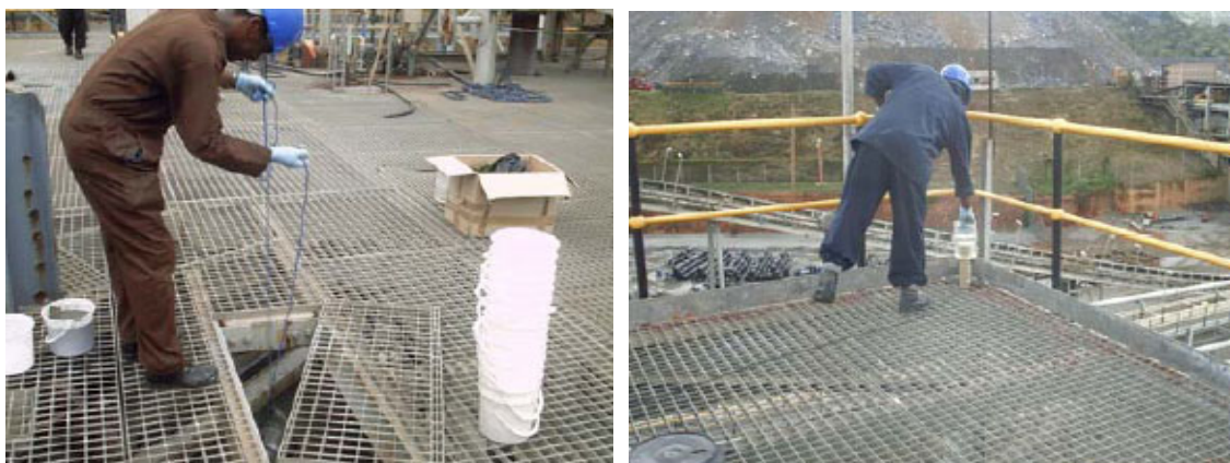
FIG. 69. Taking samples (left) and measuring them with Marineli can on top of NaI detector (left)
