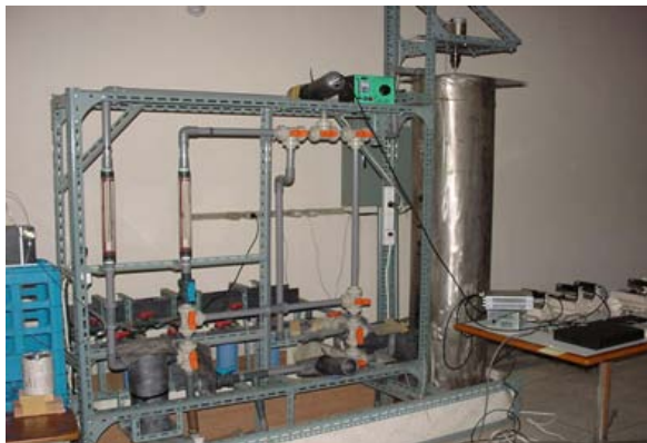
FIG. 137. Laboratory flow rig for exercising radiotracer tests.
