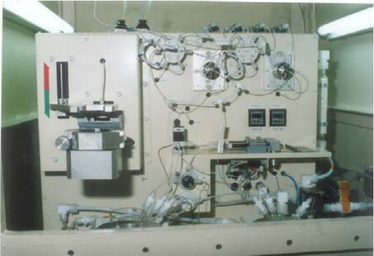
FIG. 5. Automatic synthesizer and HPLC-apparatus inside a hot-cell.
