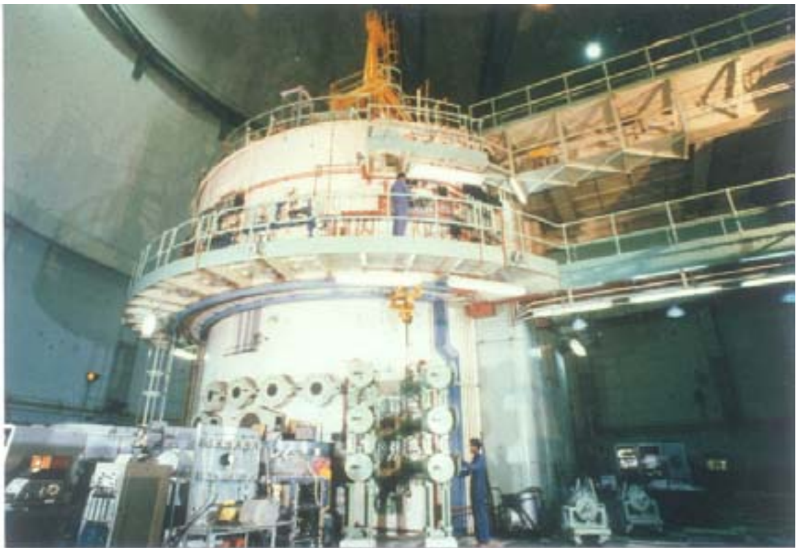
FIG. 1-2. The reactor block of a tank type reactor with irradiation facilities.
