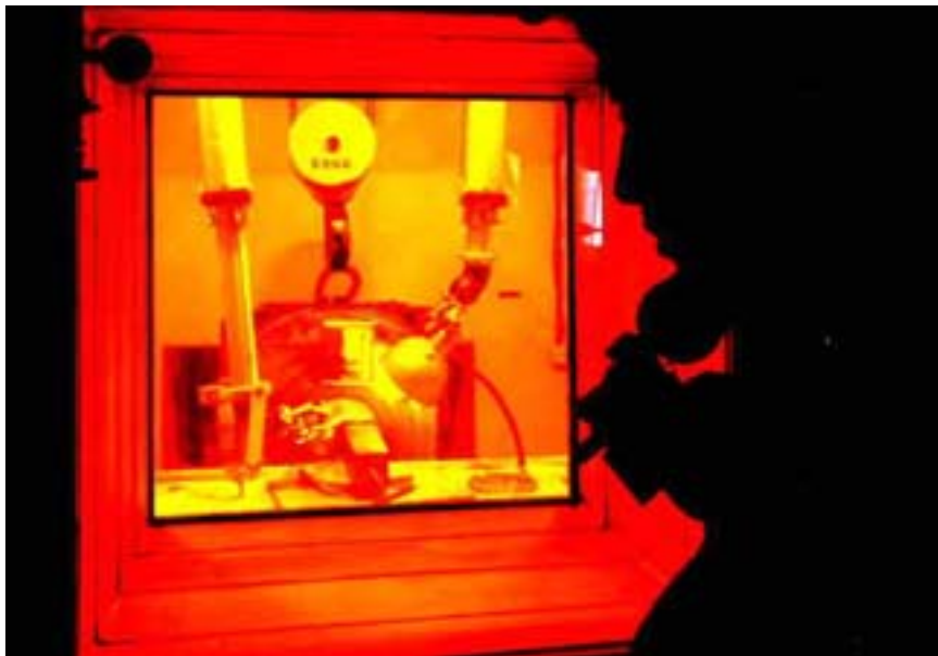
FIG. 2. Hot cell for Co-60 handling.
