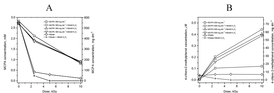
FIG. 25. Decomposition of MCPA (A) and formation of 4-chloro-2-methylphenol (B) during irradiation of solution 500 mg mg dm -3 MCPA (□), 500 mg mg dm -3 MCPA with 19 mM H_2O_2 (○), 500 mg mg dm -3 MCPA with 39 mM H_2O_2 (Δ), 500 mg dm -3 1 MCPA with 58 mM H_2O_2 (∇), waste (◇), waste with 39 mM H_2O_2 (+).
