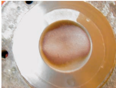
FIG. 7.4. An example of silver colloid being deposited from solution inside the front foil of a water target.
