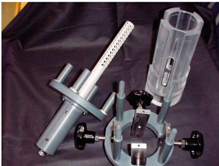
FIG. 6.2. Plating chamber for plating four targets simultaneously. The materials of construction are Lucite for the bath and various plastics for the other elements.
