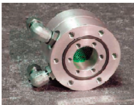
FIG. 5.7. Photograph of ^{18}\text{O} water target at the PULSAR linac from AccSys Technology, Inc. Note the grid covering the front foil to enable the latter to withstand higher pressures and beam currents.
