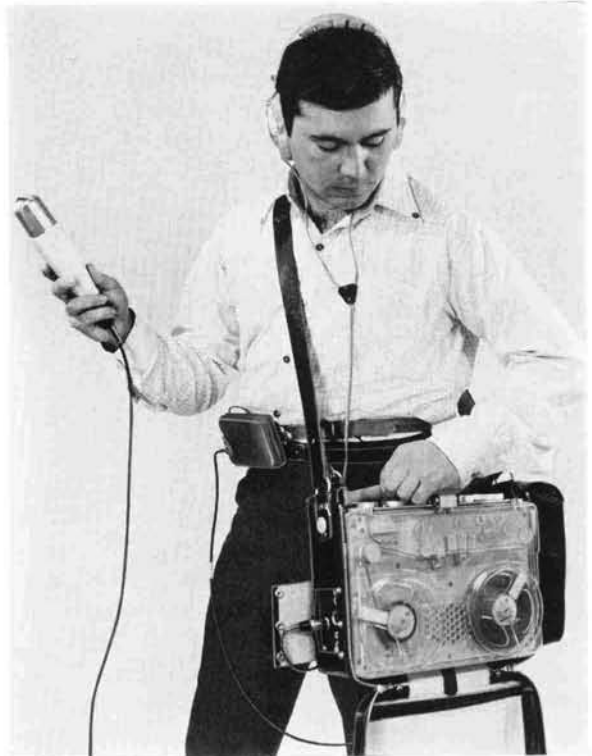
Synchronous double-system picture-sound recording without cable connections between camera and tape recorder
