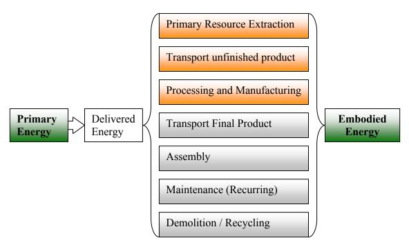
Figure 1: Breakdown of embodied energy calculations. Most embodied energy figures for specific materials are quoted using a "cradle to gate" boundary (includes orange boxes). Consumers must also consider transport, assembly, maintenance and demolition components of embodied energy. In addition, care should be taken to ensure that primary energy consumption is calculated, not delivered energy (which will understate the real energy cost).
