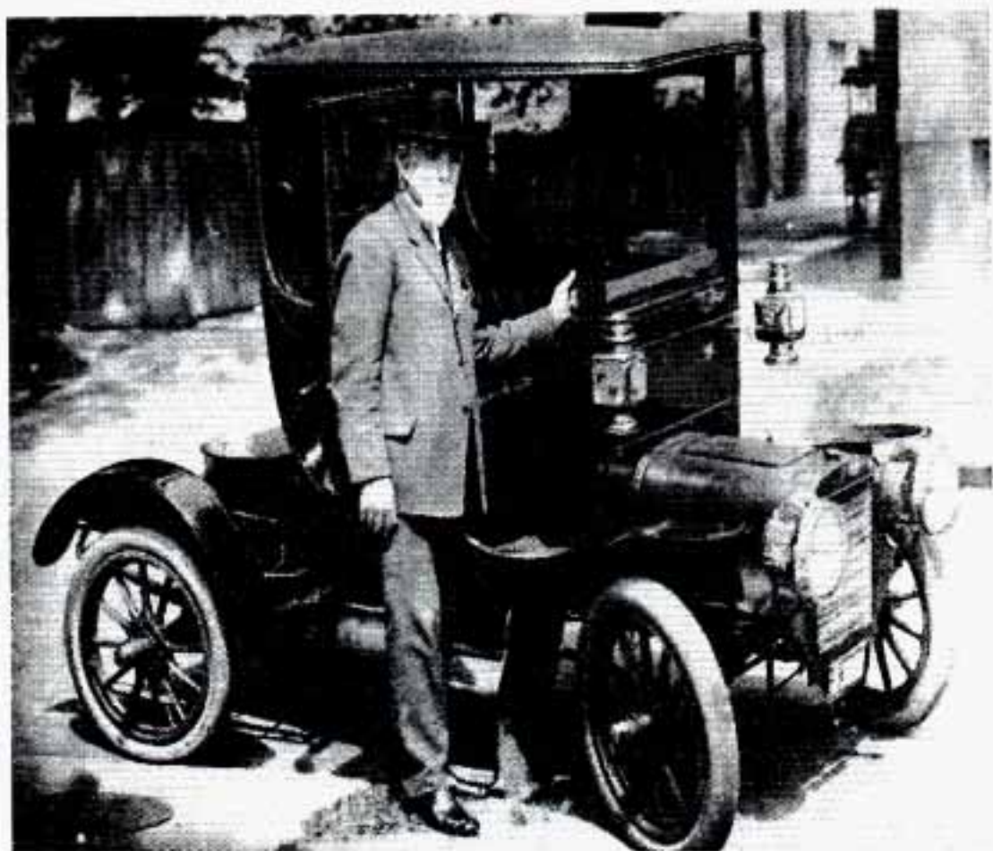
Henry M. Leland, founder of Cadillac, stands beside the 1905 "Osceola" which was built to evaluate the feasibility of a closed bodied car.
