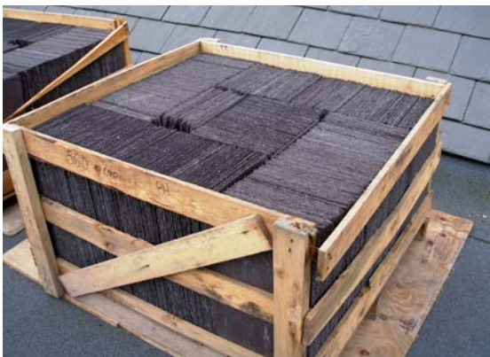
Crate of new Welsh slates ready for use. Detail of cast-iron gutter and roof valley before & after repair.
