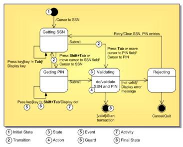
States are depicted as rounded rectangles. Transitions are arrows from one state to another. Events or conditions that trigger transitions are written next to the arrows. This diagram has two self-transitions: Getting SSN and Getting PIN. The initial state (shown as a black circle) is a dummy to start the action. Final states are also dummy states that terminate the action.
