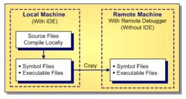
Source files are compiled using the IDE on the local machine. The executable files and symbol files produced after compilation must be copied to the remote machine.
