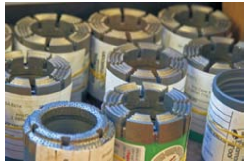
Figure 4. Diamond-impregnated drilling bits enable the ANDRILL drilling system to recover high-quality core, with up to 98% core recovery through glacial and glacimarine sediments.
