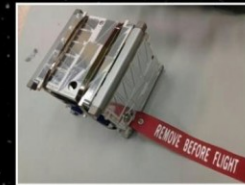
TechEdSat with the Remove Before Flight pin installed
