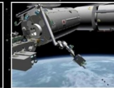
Japan Aerospace Exploration Agency (JAXA) JEM Remote Manipulator System with the J-SSOD's deploying CubeSats
