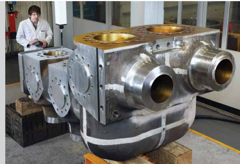
Reverse engineered main steam valve.
