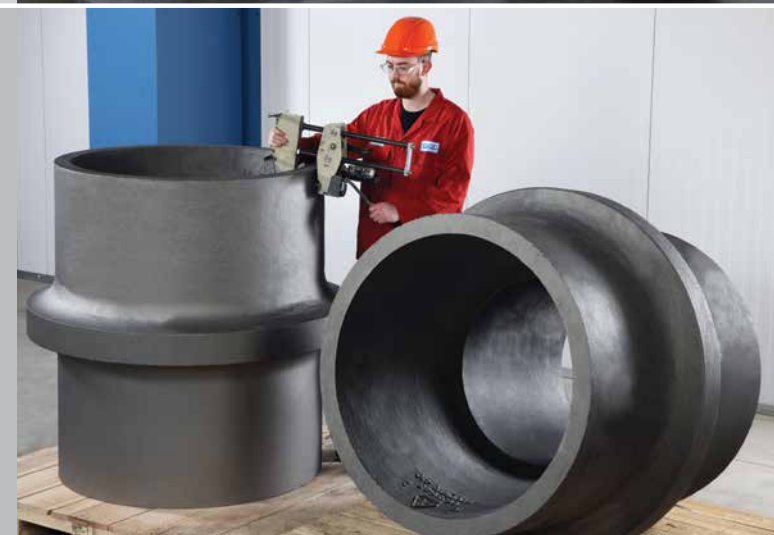
Kingpost casting for cable laying vessel.
