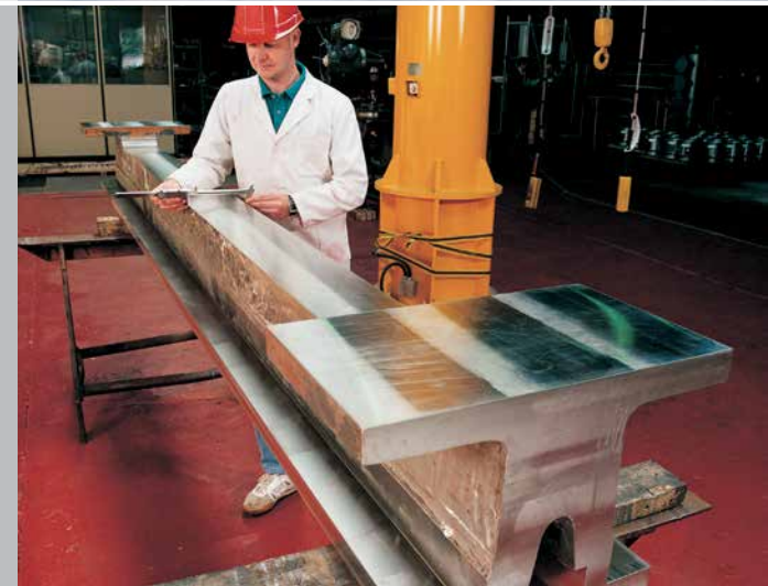
Goodwin produced 120 fully machined stainless steel guide rails to meet the specified stringent tolerance requirements.
