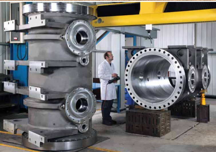
Water cooling valves for the Toshiba Westinghouse AP1000 Nuclear Power Plant.
