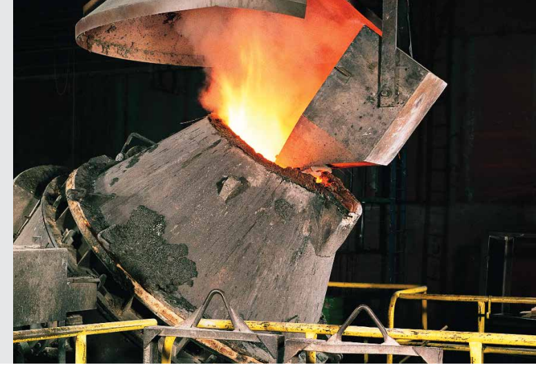
AOD refining vessel
