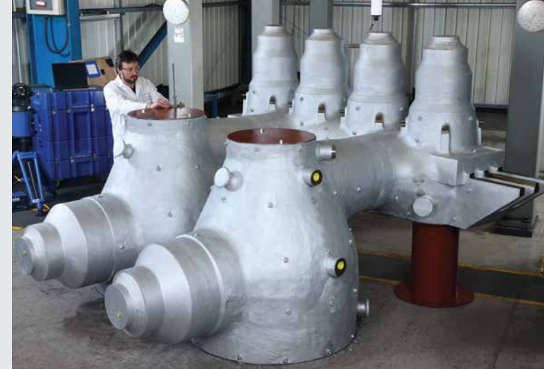
600MW control valve assembly for power generation.
