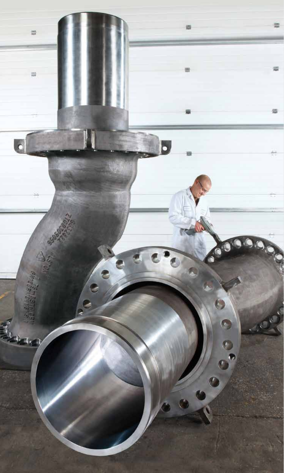
9.5% Cr fabricated pipes.
