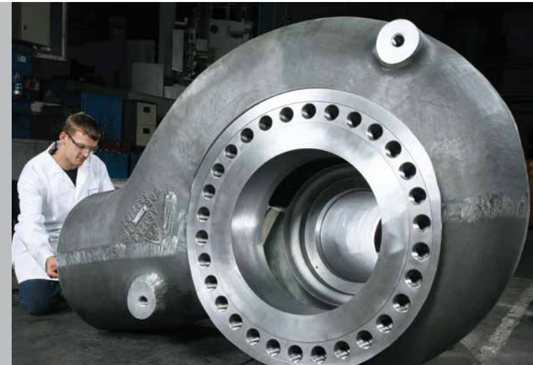
Re-circulating pump to ASME requirement.
