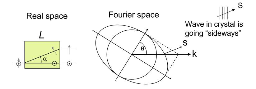
Separates polarizations with very high isolation (limited only by crystal scatter). Emerging polarizations are parallel to a very high degree since the crystal can be flat to an arc-second.
