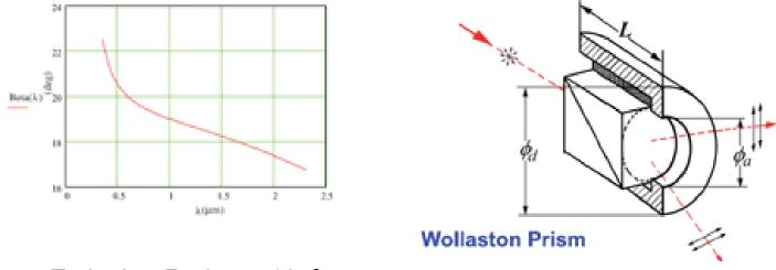
Extinsion Ratio: 5x10 <sup>-6</sup> Beam Separation Angle:16.7-22.5 at 980nm
