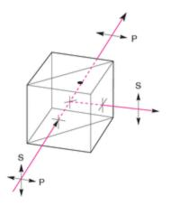
NOTE: To avoid damage, beam must enter prism on the side marked with a dot.
