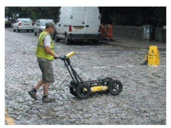
Ground Penetrating Radar survey in progress
