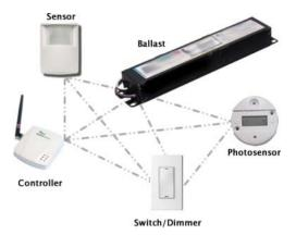
The mesh network is self-healing, in that if any disruption occurs within the network (such as a device failing or being removed), data is automatically re-routed. The built-in redundancy of having multiple pathways available helps to make the mesh network both robust and reliable.
