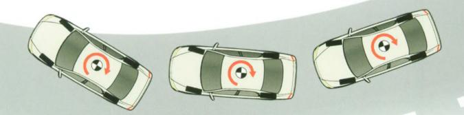
A rigid body is a prerequisite for stability, safety and comfort. The front and rear suspensions must be rigidly connected to one another through the body in order to achieve top-class road characteristics.
