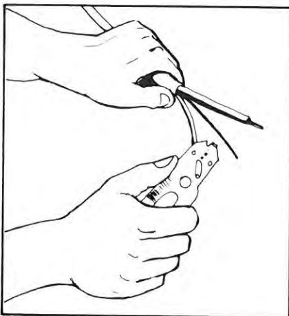
Fig. 11-15. Use wire stripper for removing insulation from smaller wire sizes. Match stripper notch to wire size.
