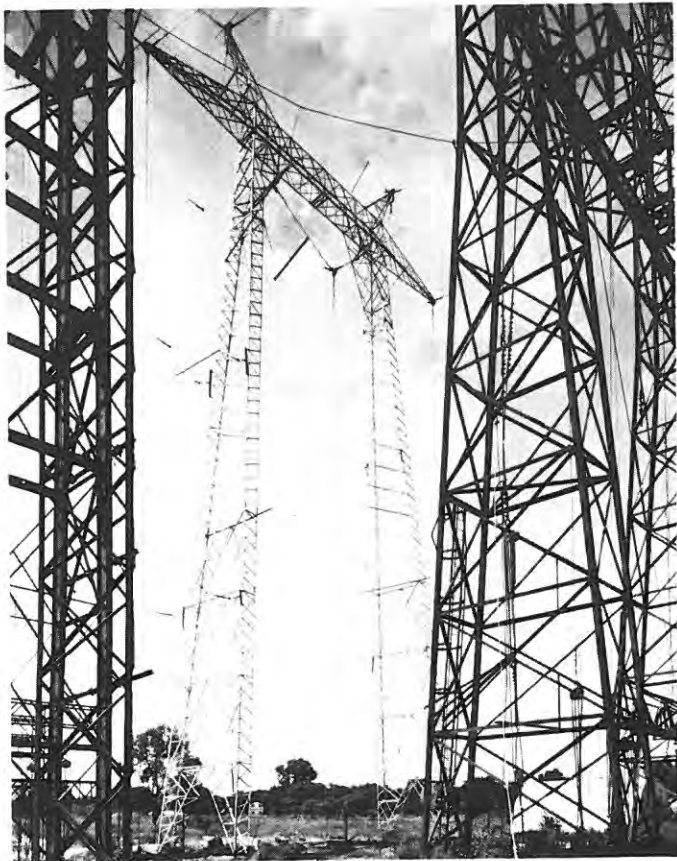
Fig. 18-10. Pacific Gas & Electric Company 500 kV "internally" guyed structure in the test rack at Adelphon, Inc. Fort Worth, Texas.
