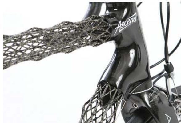
FIGURE 17. Isotruss open composite architecture [77].
