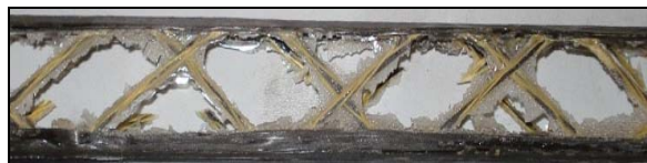
FIGURE 19. Excess resin forms a thin film between yarns.
