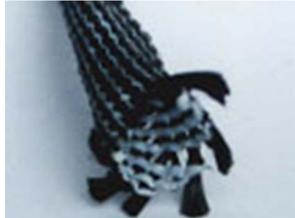
FIGURE 15. True Triaxial Braided Bearing: inner yarns are Teflon®; outer yarns are carbon fiber.
