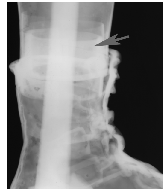
FIGURE 9.27. Radiograph of the right foot. The iron armature is visible as a wide white line in the center of the foot. A metal collar (indicated with an arrow) joins the calf to the shoe.
