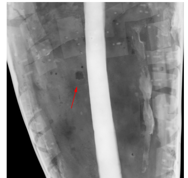
FIGURE 9.30. Radiograph of left thigh showing the larger square opening that may be a result of a trunnion or core extension. The wide white line is the iron armature, and the brass straps can be seen along the sides of the thigh.
