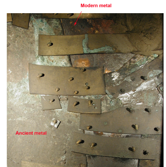
FIGURE 9.11. Interior photograph of torso taken with a hand-held digital camera showing the difference between the ancient metal and the restoration metal
