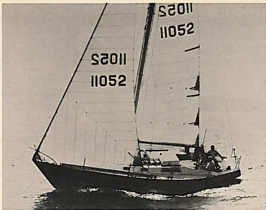
Pearson's newest. The Pearson 36 sloop, designed by Bill Shaw, is 29 feet, two inches along the waterline, 11 feet in beam, sleeps seven and features a permanent navigation center and convertible dinette. It will be featured at the 63rd National Boat Show, January 26-February 4, at the Coliseum, New York City.
