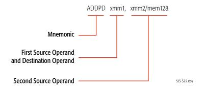
Figure 2-16. Syntax for Typical Two-Operand Instruction
