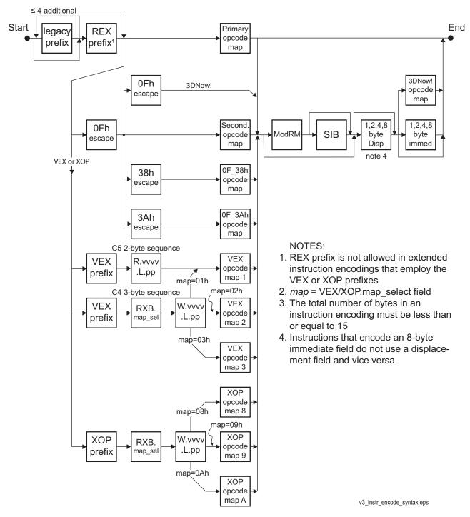
Figure 1-1. Instruction Encoding Syntax
