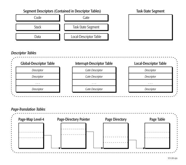
Figure 2-7. System Data Structures
