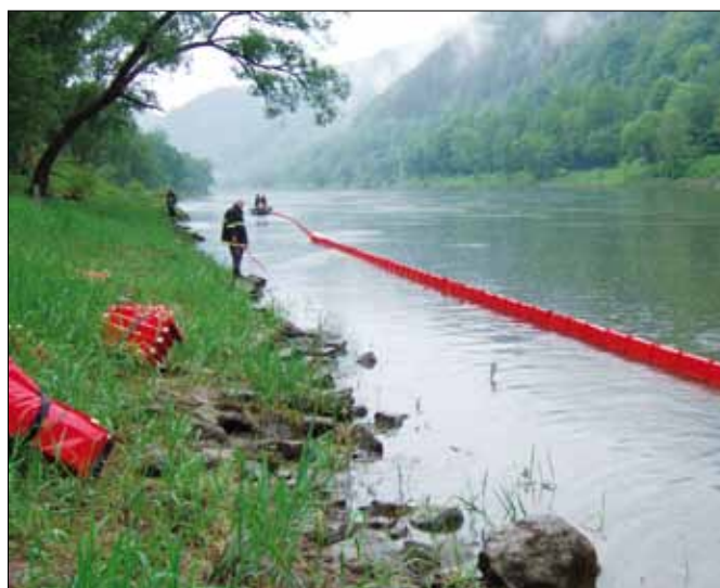
The test of patented spill containment boom REO756 took place on 6th of May 2009 in Hřensko together with fire rescue department, volunteer fire brigade and basin of Labe. Containment boom was installed manually without use of mechanization. It was fully stable and functional in flowing 0,8 m/sec. The widest river till now was over bridged with containment boom REO756. Thanks to this Czech record was created in length of installation of containment boom – 220 m.
