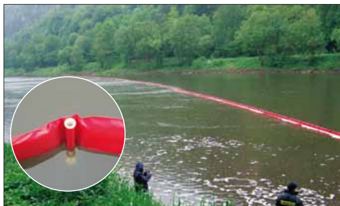
The test of patented spill containment boom REO756 took place on 6th of May 2009 in Hřensko together with fire rescue department, volunteer fire brigade and basin of Labe. Containment boom was installed manually without use of mechanization. It was fully stable and functional in flowing 0,8 m/sec. The widest river till now was over bridged with containment boom REO756. Thanks to this Czech record was created in length of installation of containment boom – 220 m.
