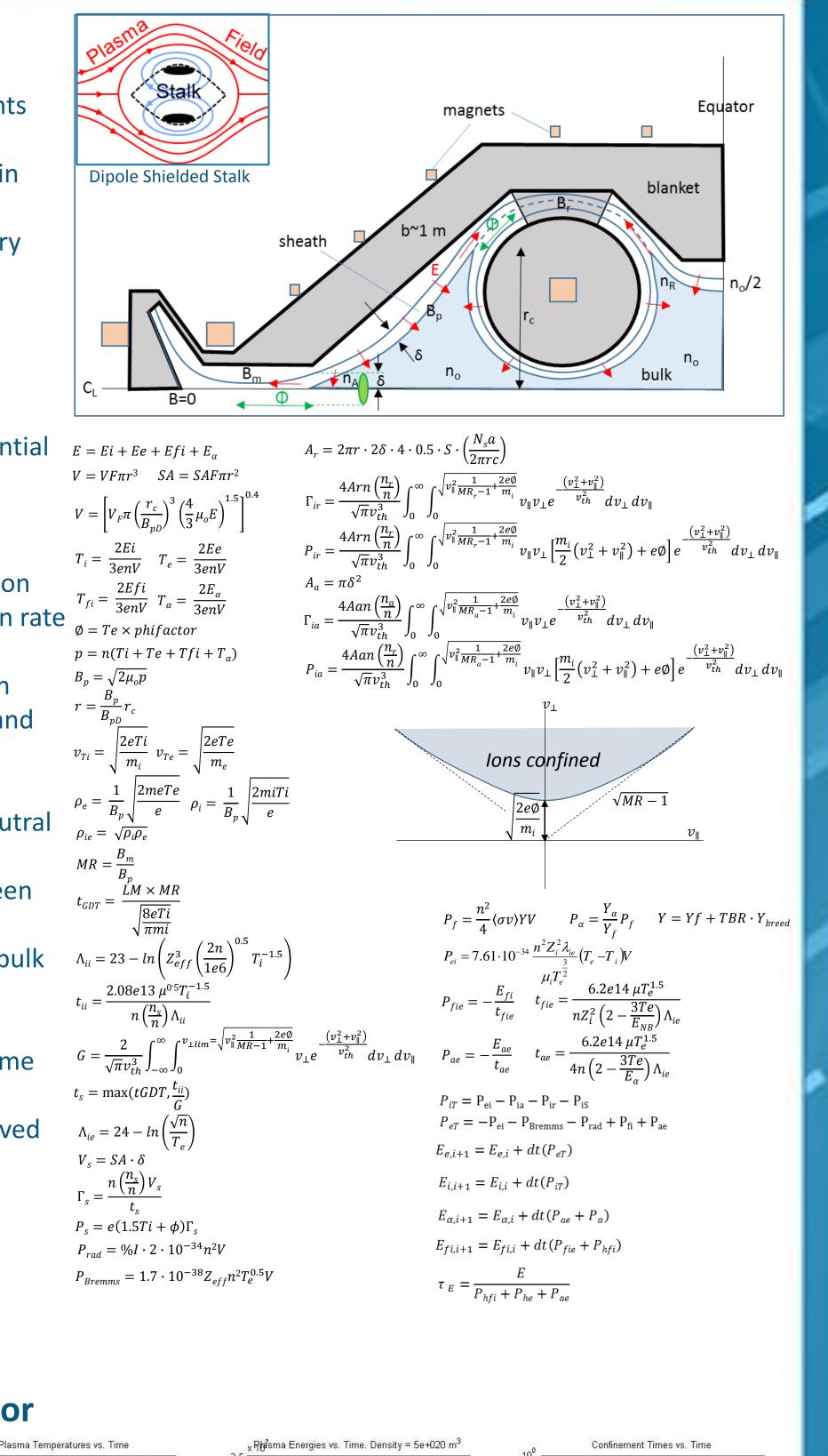
• Ring cusp loss = 8.3 MW, Assumes 5% shielding,  $n_R/n = 0.1$ • Axial cusp loss =1.1 MW,  $n_{\Lambda}/n = 0.1$ • Total Radiation = 20.8 MW, Assumes 1% Z=8 impurities • 4.2 MW/m<sup>2</sup> neutron surface heating rate • Total losses = Alpha heating power = 51 MW
