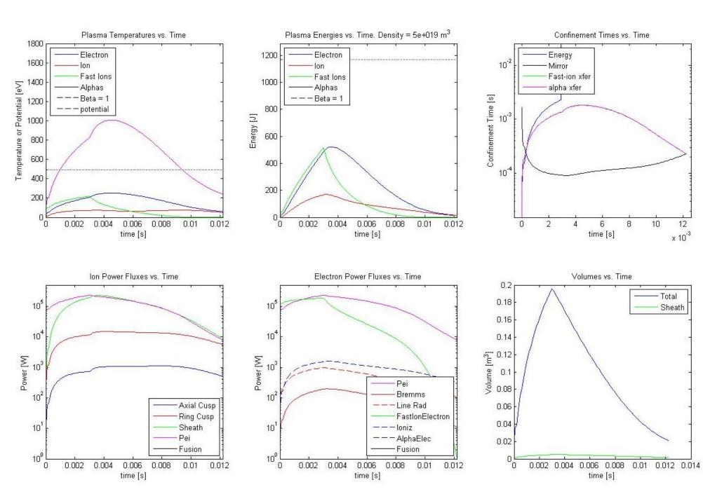
The T4B Experiment with moderate levels of neutral beam heating should show good confinement and millisecond duration plasmas, dominated by sheath losses.
