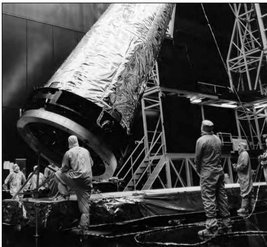
Figure 4–36. Chandra Optical Bench Assembly at TRW. (Northrop Grumman Space Technology)
