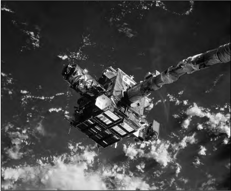
Figure 4-76. The SPARTAN 201-04 Satellite, held in the grasp of the Space Shuttle Columbia's Remote Manipulator System Arm, is backdropped over white clouds and blue waters of the Pacific Ocean. The photo was taken during STS-87. (NASA Photo No. STS087-706-020)
