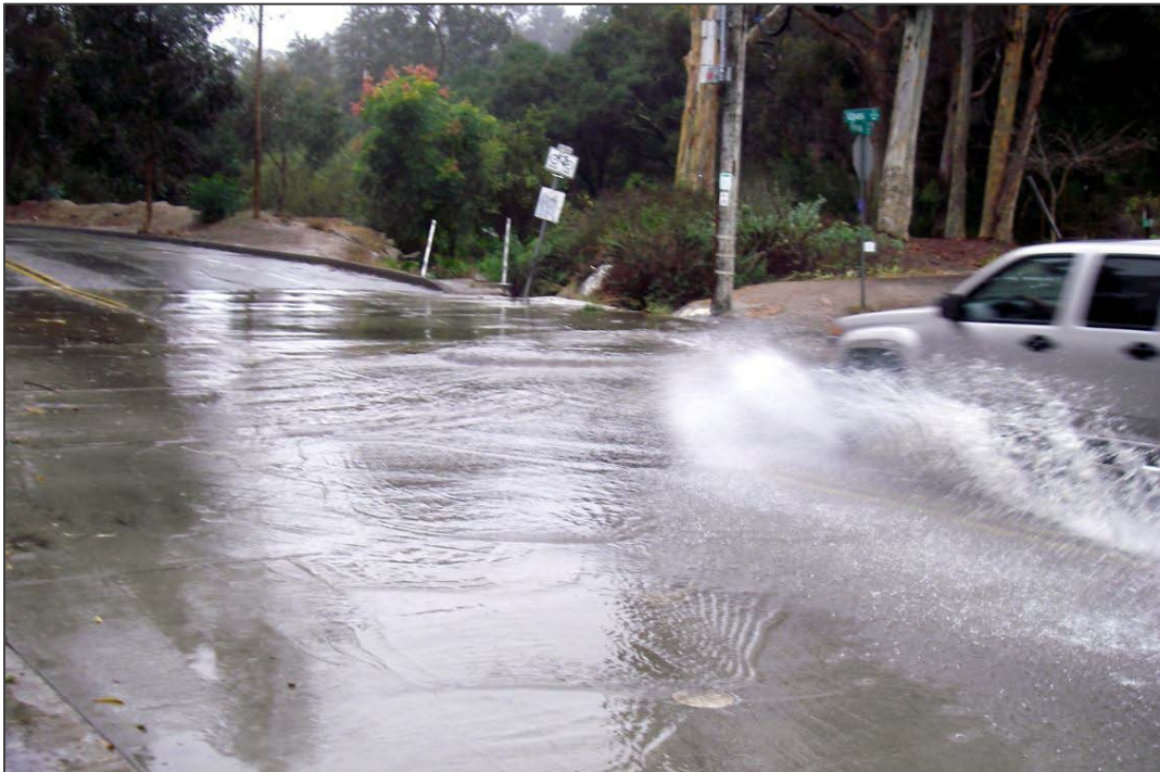
Figure 5. Winter rain flowing down Upas Street and into Florida Canyon (North Park). Winter rains have to find a way off the developed, impervious mesas. The city's storm water system uses the canyons as a drainage network.
