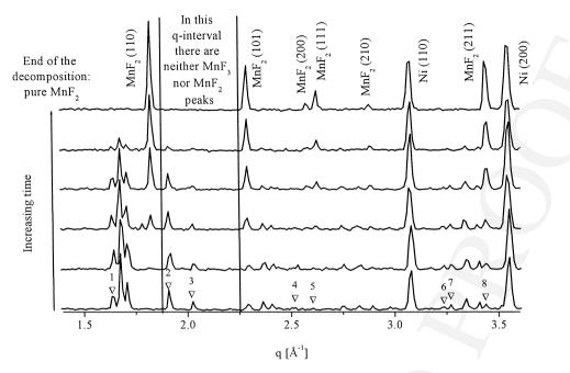
Fig. 2. A selection of the diffraction patterns collected during thermal decomposition ( $T_d = 620^{\circ}$ C, time of decomposition  $\sim 3$  h). The peaks indicated by progressive numbers can be assigned to the following Mn<sub>2</sub>F<sub>5</sub> Bragg reflections: 1 (4 0 0), 2 (2 2 0), 3 (0 0 2), 4 (3 1 2), 5 (5 2 0), 6 (4 3 1), 7 (8 0 0), 8 (4 0 3).
