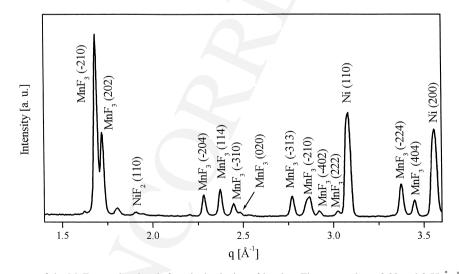
Fig. 1. Reference diffractogram of the MnF<sub>3</sub> sample taken before the beginning of heating. The two peaks at 3.08 and 3.55  $\text{\AA}^{-1}$  are produced by the Ni sample holder, the peak at 1.90  $\text{\AA}^{-1}$  is due to NiF<sub>2</sub>(s) formed on the surface of the capillary during passivation. The two peaks at 1.61 and 1.80  $\text{\AA}^{-1}$  are probably produced by impurities.
