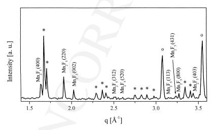
Fig. 3. Detailed view of the first (lowest) diffractogram of Fig. 2, which shows the onset of new peaks. To these new peaks Miller indexes of  $Mn_2F_5$  reflections are assigned. The remaining reflections due to  $MnF_3$  and to the Ni capillary are indicated by asterisks and circles, respectively.
