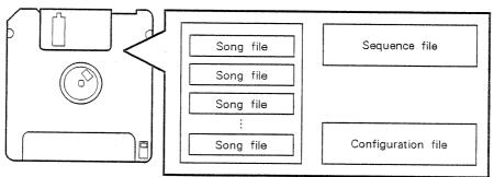
If, when SUPER - MRP is started up, you insert a song disk that contains a sequence file, the sequence file / song files (Bank A) / configuration file will be loaded into memory automatically. Then simply press PLAY and the songs will playback as specified by the SUPER - MRP settings. Of course even after SUPER - MRP is started up, you can exchange disks and play.
