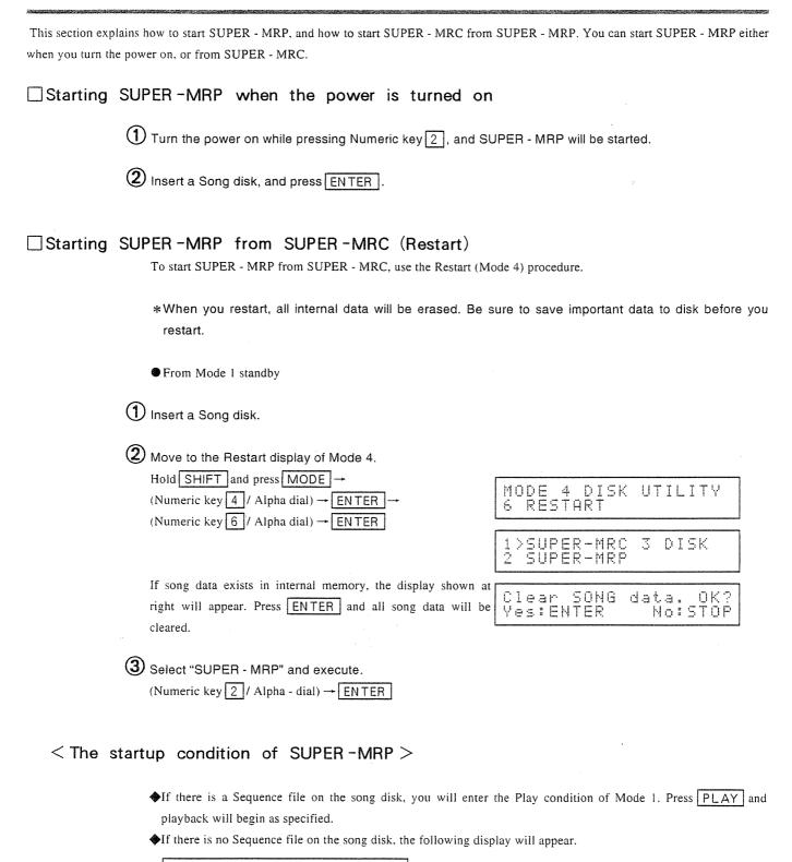
Press STOP to get the mode select display (Mode 2 display). To create sequence data, press ENTER ( P.181).
