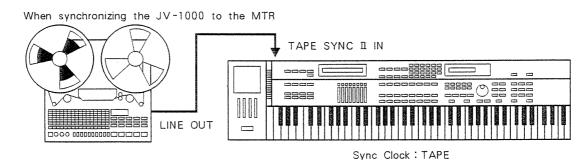
To synchronize the JV - 1000 to the MTR, set the sync clock ( P. 62)) to "TAPE". Playback will start when the tape sync signal is received from the TAPE SYNC II IN jack.
