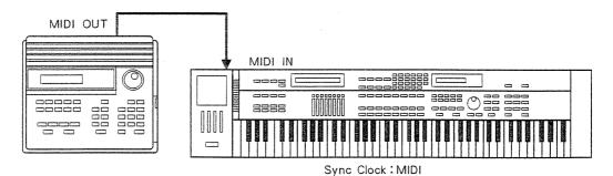
When playback is started with the JV - 1000 sequencer, the MIDI clock will be transmitted according to the tempo. The JV - 1000 will be operating its own clock at this time, so it will ignore any MIDI clocks received from an external source. When using the JV - 1000 as the slave, set the sync clock ( P. 62) to "MIDI". When set to "MIDI", playback will start when the start message and MIDI clock is received from the MIDI IN.
