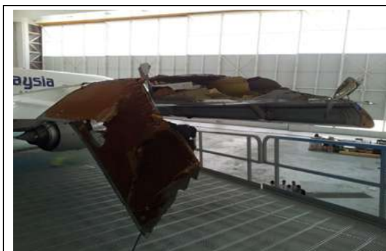
Figure 1.6A - Right Wing Tip Damage
