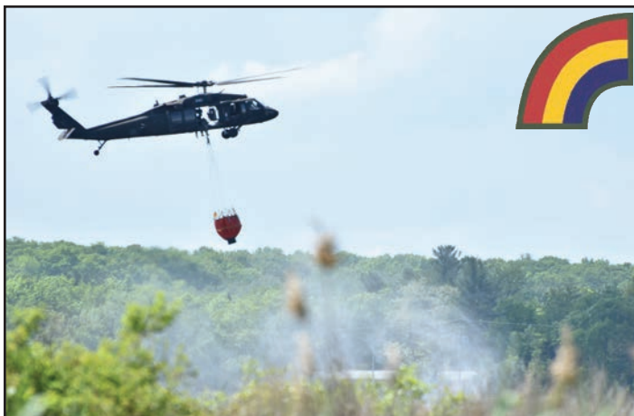
New York Army National Guard aircrew from the 3rd Battalion, 142nd Aviation prepare to fill a Bambi Bucket with water from Round Lake, N.Y., May 31, 2017. The aviators were conducting a slow pick-up in order to fill their bucket with as much water as possible.
