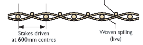
Figure 4.1.1 PROFILE OF SPILING REVETMENT
