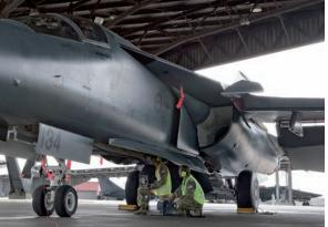
Loading cameras into the RF-111 sensor bay
