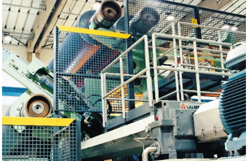
This roll cylinder drive is part of a mechanical drive system delivered for Aylesford's PM 14.
