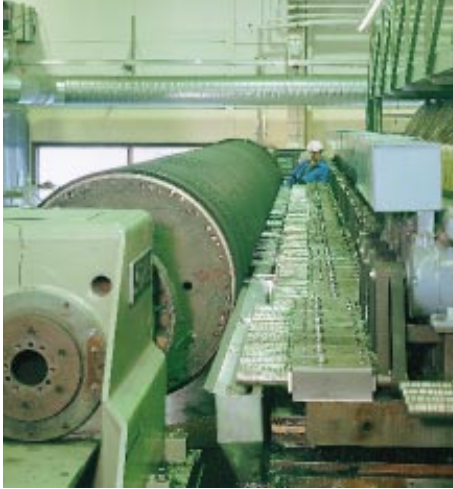
A paper machine roll waiting for drilling, following covering with rubber at the Oulu Rubber Factory.
