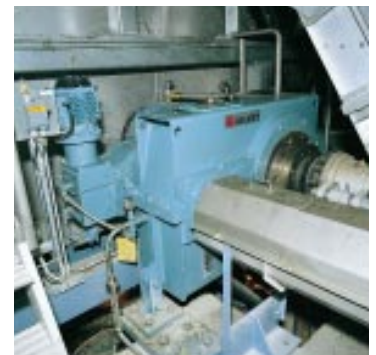
A drive developed for Valmet Yankee cylinders improves machine runnability.
