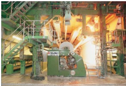
In January 1996, the Central Laboratory's Optiblade coater reached a record speed of 2,503 m/min. The photo shows an Optiblade coater for LWC paper grades, delivered to UPM-Kymmene's Kaukas mill.
