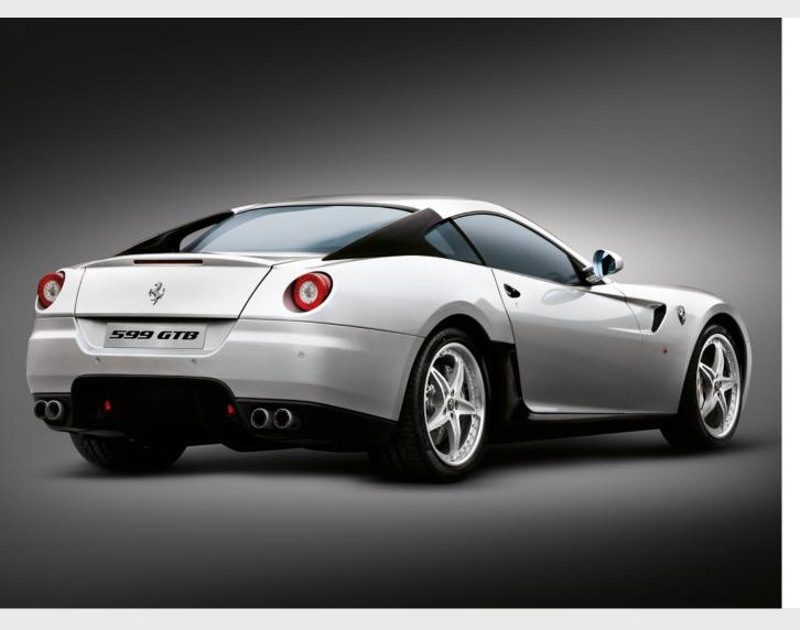
The aerodynamic fins are the side view's most distinguishing characteristic and technically speaking, their contribution is vital for achieving the aerodynamic load goals required at high speed since they channel and maximize the air flow towards the nolder. Using exposed carbon fiber has reduced the component's weight by 50% while maintaining the same aerodynamic efficiency.
