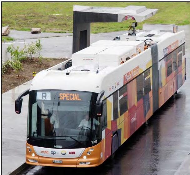
Figure 11.3 Electric bus recharging (Geneva)
