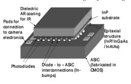
Figure 3. Outline of Infrared Image Sensor based on InGaAs photodiodes.
