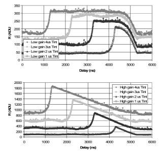
Figure 6. Photo response of pixel to a 20 ns long light pulse incident on imager at different delays with regard to the camera trigger pulse. A longer delay means a later light pulse. The curves are slightly offset with longer exposure times in higher positions.
