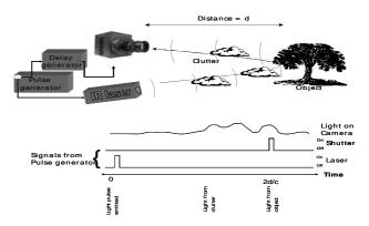
Figure 1. Example of gated imaging with pulsed laser: A tree is partially obscured by mist or other clutter that reflects light and reduces the contrast in the image of the tree. The electronic shutter of the camera is kept closed (i.e. the camera is not integrating light) during the time that the light from the clutter is incident. The shutter is opened only at the time of incidence of the light from the tree.
