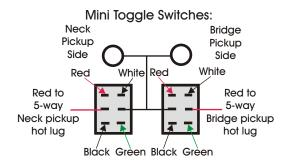
Note: Solder Ring Terminal Grounding tabs together to common ground of mini-toggle switches.
