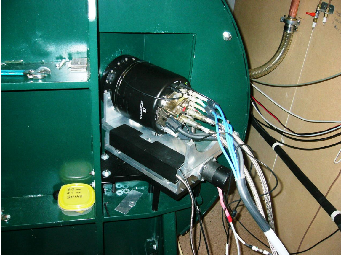
New 4k by 4k Spectral Instruments CCD camera mounted on the Hercules spectrograph
