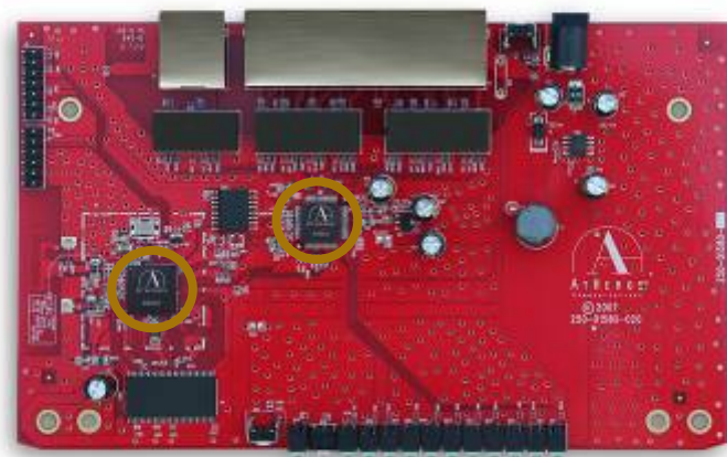
AR5007 Single-Chip 11g Solution + AR8216 10/100 Ethernet Switch
