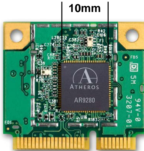
Atheros 130nm QFN Package 10 \times 10 = 100 \text{ mm}^2
