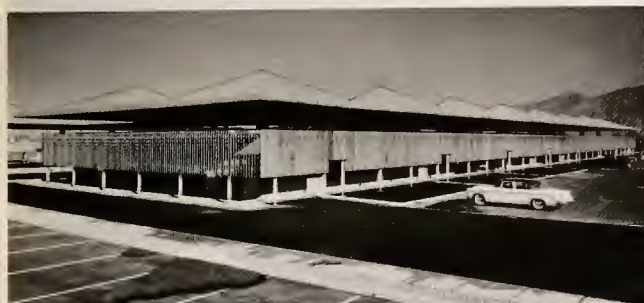
EXCITING NEW SHAPE in buildings features Wilmot Medical Center, built at Tucson and partly owned by Webb Corporation. Opened in October, it has a 36-point hyperbolic paraboloid form roof which is a separate, parasol-like shelter for offices below. Center has space for 60 doctors, dentists and opticians; a pharmacy, optical dispensary, physical therapist, medical laboratory and diagnostic X-ray lab.
