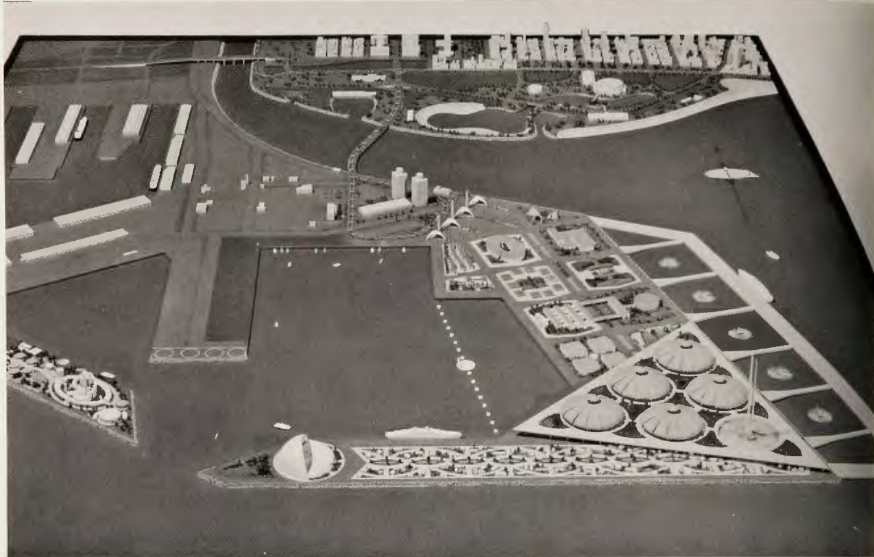
SITE PLANNING for the Long Beach World's Fair of 1966 is shown in the impressive model pictured above, the creation of the Aetron Division of Aerojet-General Corp. Part of the city of Long Beach is shown at top of photo. Exposition will rise on man-made island and exposition buildings will cover much of 320 acres. Ocean liners will be able to dock beside the fair site.
