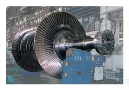
The development of longer last stage blades for steam turbines is one of the most effective solutions to achieve a compact and highly efficient turbine design at large unit capacities. As such, Hitachi has successfully developed multiple kinds of long last stage blades based on its own proven technology and processes.
