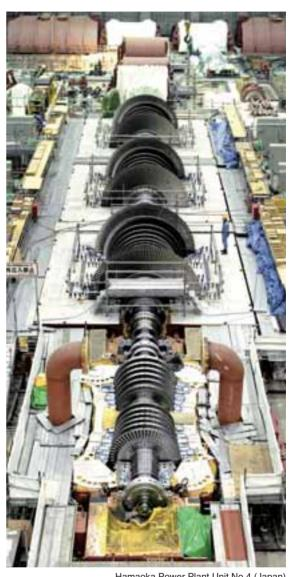
Hamaoka Power Plant Unit No.4 (Japan) 1137 MW, TC6F-43, 1800rpm 6.55 MPa, 282/251°C
