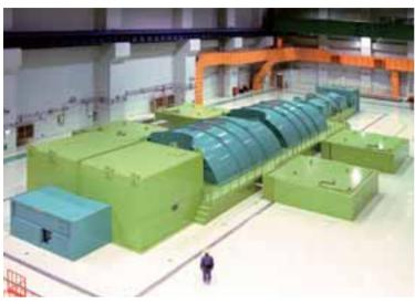
Shika Power Plant Unit No.1 (Japan) 540 MW, TC4F-38, 1800rpm 6.55 MPa, 282°C
